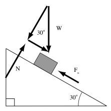
For sliding to happen a force of half the weight must be able to overcome the force of static friction. The maximum value of the force of static friction is equal to the product of  $\mu_s$  (the coefficient of static friction) and the normal force, which equals in magnitude the component of the block's weight perpendicular to the plane. This perpendicular component is equal to the product of cos 30° and the weight. In other words, the following is the condition of sliding:
