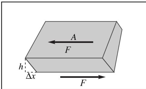
The **shear modulus** describes the type of deformation, pictured at lower left, which occurs when an object is subjected to a tangential force on one of its faces while the other is held in a fixed position. The *shear stress* is computed by taking the ratio of the force applied to the area of one of the faces. The *shear strain* is the ratio of the horizontal distance the sheared face moves to the height of the object.
